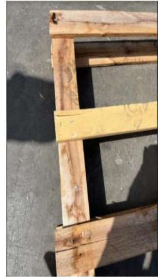
Figure 7 Wood Pallet with small broken edges that cut the bumper's cover
