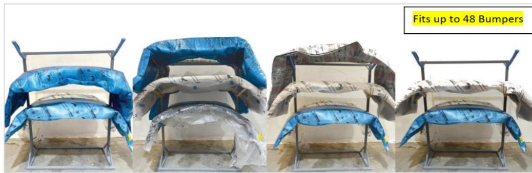
Figure 18 New storage racks with bumpers on
